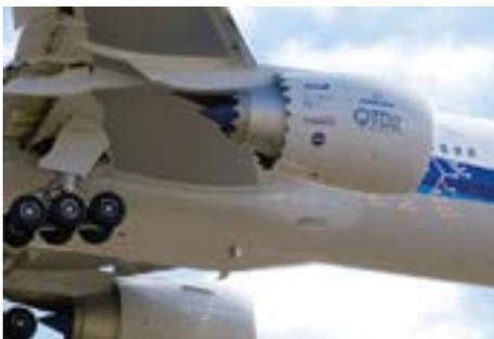
*Testing on this All Nippon Airways 777-300ER showed that the chevron shape of the engine nozzle helps reduce noise. © Boeing. All Rights Reserved.*
