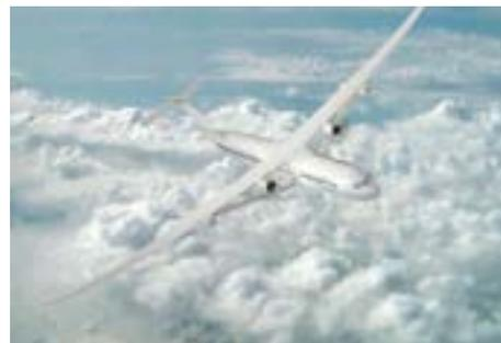
Another experimental green aircraft currently in development by Boeing is SUGAR Volt. It is a hybrid electric and jet fuel plane, similar to the hybrid cars we drive today that use both electricity and gasoline. SUGAR stands for Subsonic Ultra-Green Aircraft Research, a group which helps design airplane technologies needed 20 years from now to meet green aviation requirements, including fuel efficiency.
