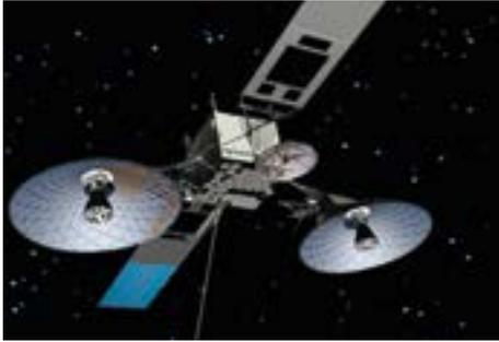
*Satellites like this Tracking and Data Relay Satellite (TDRS) have large antennae and solar panels that deploy once they are in orbit.
